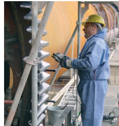
Inspection engineers making silicone rubber impressions of tooth flank damage (above) and measuring tooth thickness (below)
