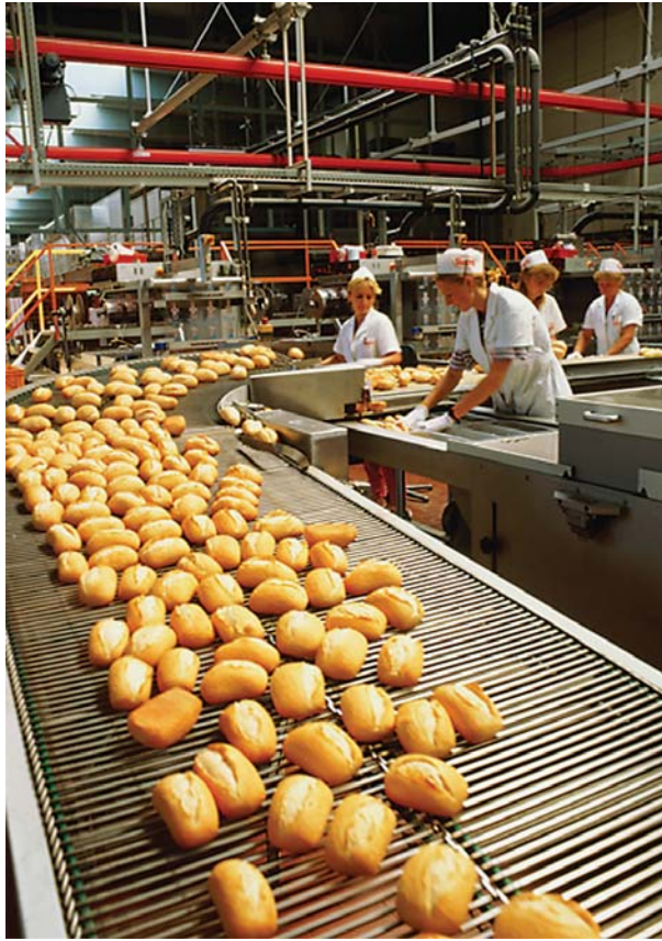
Figure 2. Conveyor Belt Operating with H1 Lubricant
