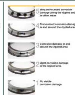
Figure 3. Corrosion grades in the rippling test
