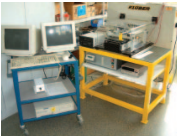
Test rig for electric contacts Determination of service life by measuring the electric resistance
