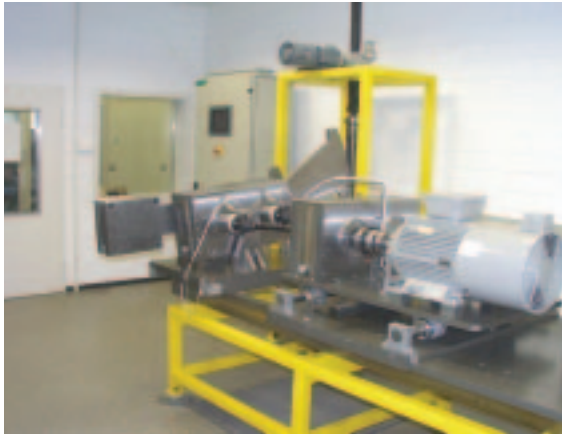
CV-joint test rig Determination of service life
