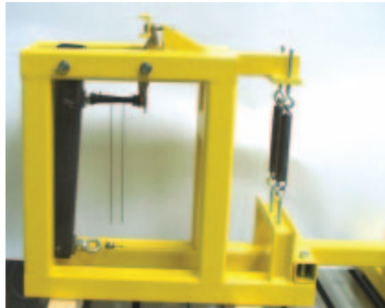
Test rig for clutch master/slave cylinder Recording creaking and squeaking noises
